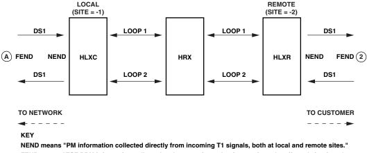
FEND means "PM information collected directly from incoming 11 signals, both at local and remote sites. FEND means "ESF PRM information collected at the opposite ends of spans from the affected circuit and returned to the system via the ESF Datalink, both at local and remote sites". The framing format must be ESF in order for FEND information to be displayed.
